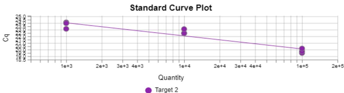
Target: Target 2 Slop: -1.965 R<sup>2</sup>: 0.896 Y-Inter: 29.931 Eff%: 222.693 Error: 0.254
